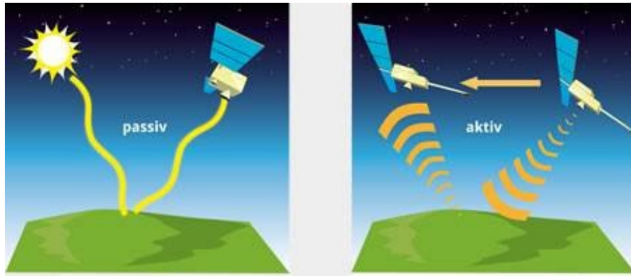
Fig. 10: Passive and active recording systems for earth observation.
