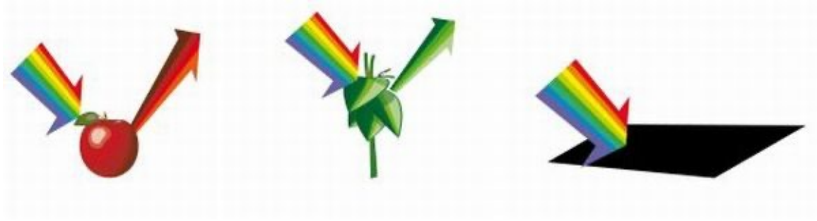
Fig. 13: Reflection and absorption.
